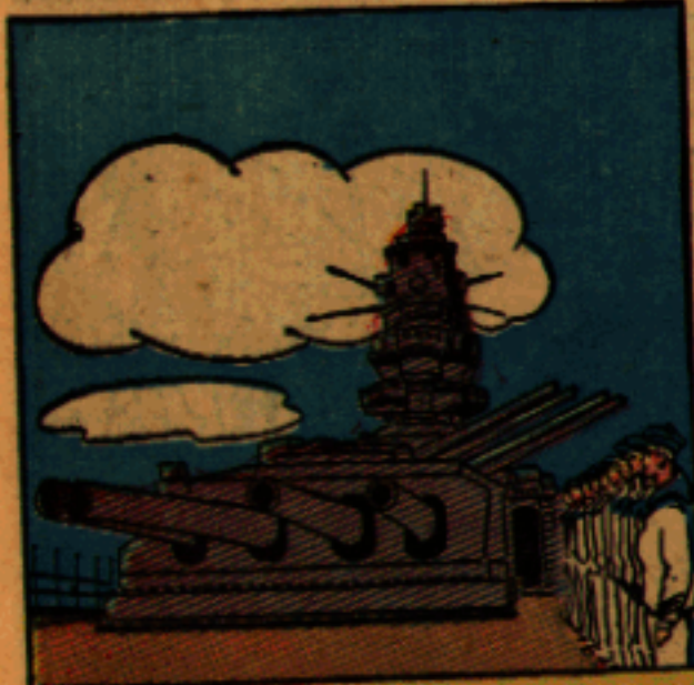
THE STRASBOURG - 25,000 TON SISTER SHIP OF THE DUNKERQUE. MOUNTS 8 13 IN. GUNS. SPEED - ABOUT 30 KNOTS.
