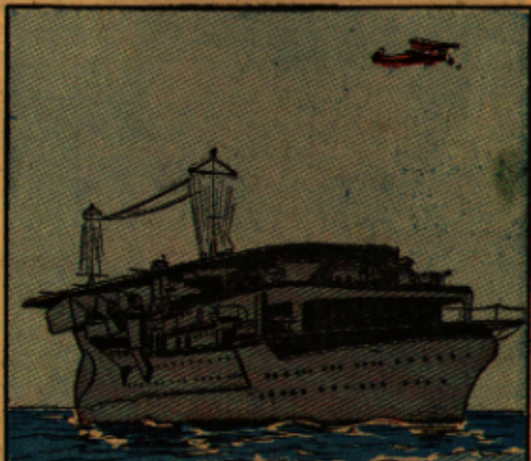
KAGA - AIRCRAFT CARRIER - 26,900 TONS, 720 FT. - TEN 8 IN. GUNS - CARRIES 60 PLANES.
