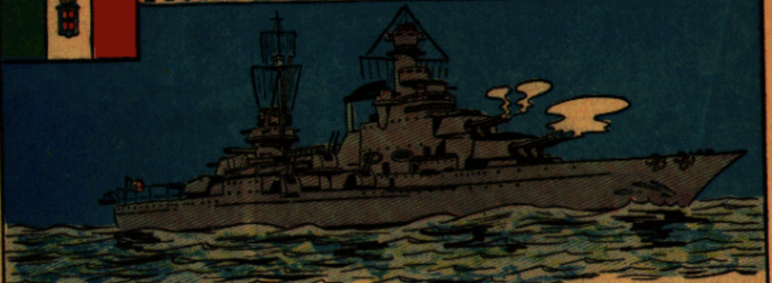
THE CAVOUR - A 35,000 TON RECONSTRUCTED BATTLESHIP, ORIGINALLY BUILT BY ITALY IN 1915 - SPEED 26 KNOTS, ARMAMENT UNKNOWN.
