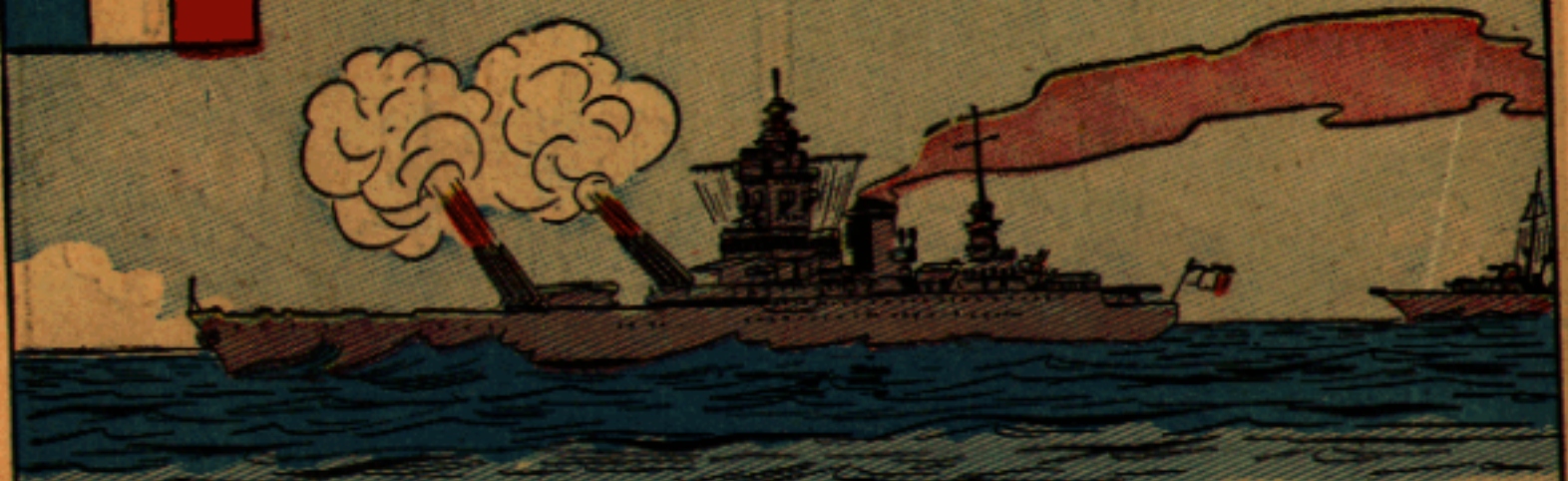
THE RICHELIEU - BIGGEST WARSHIP EVER BUILT FOR THE FRENCH NAVY. A DISPLACEMENT OF 35,000 TONS; EQUIPMENT - EIGHT 15 INCH GUNS, FIFTEEN 6-INCH GUNS, WHICH ARE USED FOR ANTI-AIRCRAFT ARMAMENT. SPEED NOT KNOWN.
