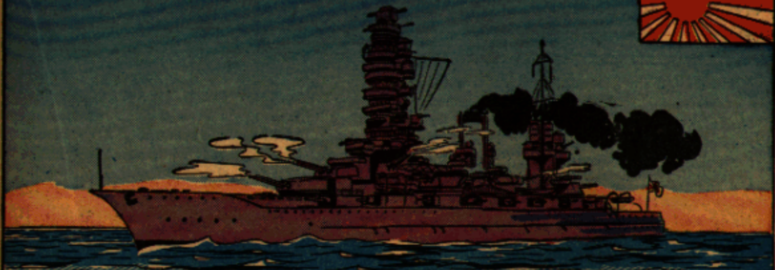
BATTLESHIP MUTU - 33,000 TONS, PLATED WITH 12 IN. ARMOR, CARRIES EIGHT 16 IN. AND 20 5.5 IN GUNS, SUPERIMPOSED. THE HUGE FOREMAST, DESIGNED TO REDUCE VIBRATION, HAS PROVEN SUCCESSFUL.
